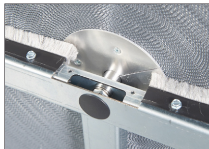
(5) Remove the brush seal and the bearing cover
