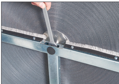
(7) Loosen the hexagon head screw
